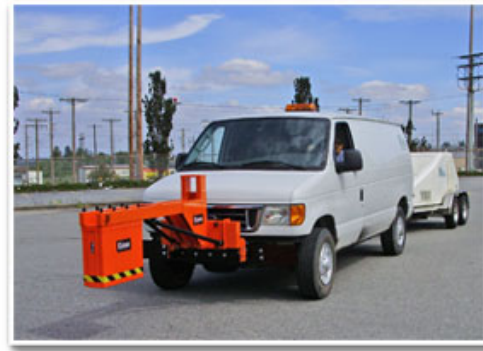
GPR (Layer Thickness, Trapped Moisture)
